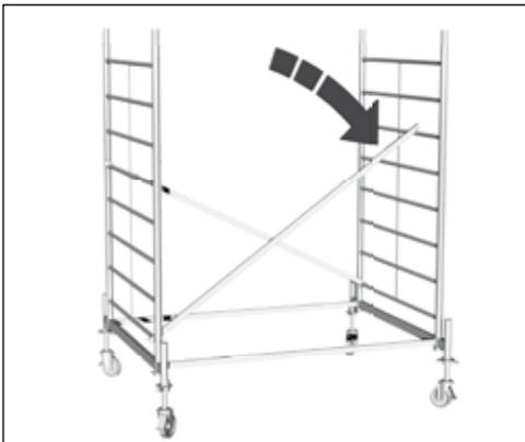
Attach the second diagonal to the fifth rung of the vertical frame to the first rung on the other side. Secure it with the securing kit.
